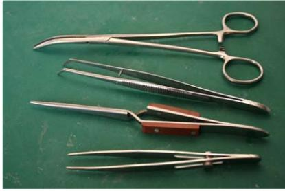
holding nuts in tight places while turning screws to engage with them. These can be bought quite cheaply at discount tool suppliers. Also shown are three kinds of tweezers. The top pair rely on hand pressure to hold the item, while the centre pair are sprung by the cross-over grip design, The tweezers at the bottom have a self-sliding lock which maintains whatever pressure is applied to them and therefore can hold small things - such as nuts and washers - quite firmly
