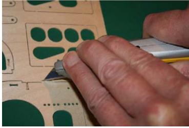
For the epoxy glass use the same 'chopping' technique as with the ply, but do it from the reverse side – ie. tab flush with the top surface.
