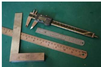
more accurate than a ruler and very useful for checking the diameter of wire and tube and so on.
