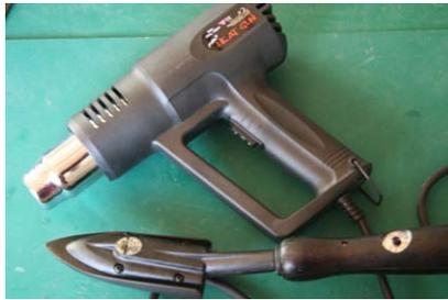
Greenfinch without using a specialist modelling Hot Air gun. However a hot air gun is useful where we make use of low temperature heat shrink tube (shrinks at 80 deg C) in the kit. However, the sealing iron can be used for this as well. (Note: DIY type heat guns sold for paint stripping are not recommended since their temperature is much too high, and not compatible with modelling materials).
