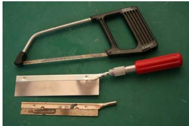
1.2.11 Hand held small drill holder. This one has a 1mm drill in one end, and a 1.7mm in the other.
