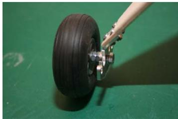
(Do it up gently finger tight, then back off one flat - ie 60°). Then lock the second nut against the first, (use two spanners for this, keeping the nut closest to the wheel stationary, and tighten the second one on to that). Check the wheel still able to rotate freely, add another four washers to give the clearance required if you are fitting spats, then insert into the axle
