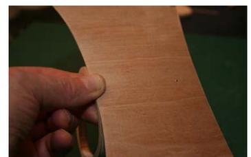
up the parallel lines and help you to keep MC1 square with MC2. Pull the cowl down each side of MC2, lining up the bottom edges with MC2, and arranging MC1 to fit close to the chamfered angle on MC2, and that the edge of MC1 is parallel and flush with MC2 at the top centre.
