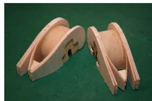
**2.46.10** The inner face of each spat has SP6 over the SP4, and then three SP7's. The outer face has five SP8's. If you've proceeded as 2.46.8, then you're now done with this stage. If you've gone with 2.46.9 then the next step is to apply resin glue to all the interleaved areas, using a brush to get it right into the
