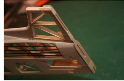
**2.42.8** Next you need a very small amount of epoxy or slow cyano, and then either: (a) apply a TINY amount to the surface of F10 in the middle of the slots – use the tip of a piece of the 1mm wire for this – one dot for the shorter slots, two for the longer ones.
