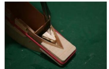
**2.46.7** First of the balsa laminations to fit is SP4, which fits up against SP1 and around SP5. If you use resin, spread it evenly with a brush, and use weights while it dries to prevent the balsa curling up. Keep the rear end pulled in with tape. Slow cyano also works well and is very quick of course, but make sure it's evenly spread out. However, cyano does tend to harden the balsa which can make carving a little more difficult, and also more rapidly takes
