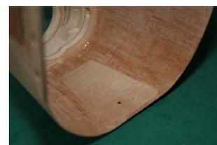
**2.43.13** These photos show the external MC1d, (shown 1.6mm thick but now 0.8mm), and the internal 0.4mm MC1e.
