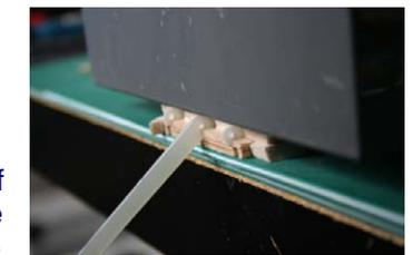
Use 5mm balsa scraps if laminating the inner face with resin after fitting the epoxy glass parts.
