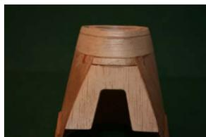
checking often to see how it's going. There is no absolute correct shape for the cowl, just try to get a smooth transition from one curve to the next. At the front the slope from the side will come
