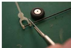
Fix the axle with a very small amount of 5 min epoxy. To do this just push the axle in a bit at one side, and place a pin heads worth of epoxy in the depression so formed, repeat the other side, return the axle to flush each side, wipe off any excess, and you're done.
