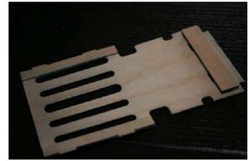
be) and then the forward sides of it engage with the slots in FS2a each side. To enable this, the rear tab FB5b has to be spaced away from FB5 by
