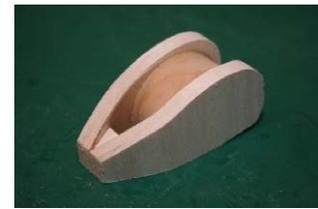
**2.46.12** The upper laminations are each made up from one longer and one shorter section. We recommend using either pva or aliphatic resin for this, (although slow cyano can be useful with a slightly modified technique – see later note). Use the longer lengths starting from the front and bending around to the flat section at the rear..
