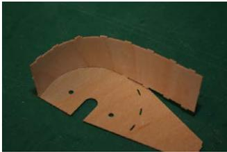
gently form it into a curve between thumb and fingers. You can see the radius required by the slots in SP1 and SP2. The inner wall of the spat chassis is SP1, lay that
