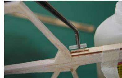
**2.42.10** Next up is the rudder. (Remember to strengthen the surface with penetrating glue). Position the rudder tubes using RHTG, making sure of course that it's the right way up! – i.e. open slot to the top and aligned right up at the top of the rudder post – this will give the correct alignment between the fin and rudder.
