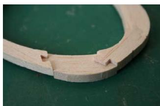
extremely important, since the sides have to be chamfered at exactly the correct angle so that the cowl MC1 will take up the
