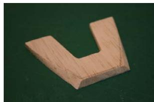
is chamfered not only because it allows cooling air to escape more easily, but it also looks better. Now glue MC9 in place. Use a slow drying glue so you have time to adjust the fit.
