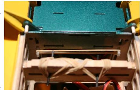
You will see a little free movement of the spring lever between the spring beam and the fuselage side. This gives the wheels a bit of realistic positive camber when in the unloaded (flying) condition. However, if you like you can damp out the free movement by using a self adhesive foam pad fixed between FS1 and the spring lever UC4.
