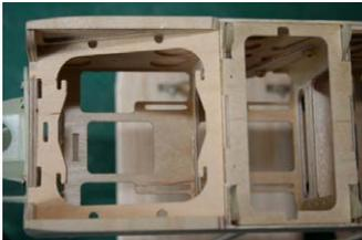
They are designed so that they can be sprung into position, using the natural flexibility of the 0.8mm ply to hold them in place without any screws springs, clamps, or magnets.
