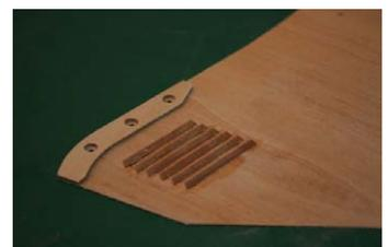
**2.43.4** Now do a trial arrangement of MC1 around MC2. Note there is an alignment notch in the centre front. Draw some parallel lines along the top edge of MC2 (photo) and note the three holes either side of the central notch, which when looked through can pick
