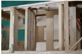
... and one covering the tank/ESC/undercarriage section, FB5.
