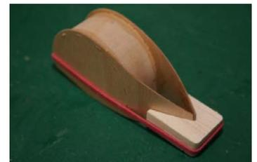
**2.46.6** Push the rear sections together into the 'V' of the SP19 jig, and use a rubber band around the assembly to hold it there. Now glue the two triangular parts SP15 into the joint, one near the top and one towards the bottom, but make sure there is space (around 1½ ~ 2mm) at the bottom to fit in the balsa cover plate SP17 flush with the base of the spat, but don't fit SP17 just yet. That completes the basic ply chassis.
