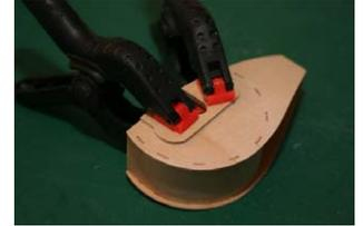
While that is drying, cut out and laminate the two 5mm balsa pieces SP19 – these parts make a jig to hold the rear of the chassis together at the correct angle.
