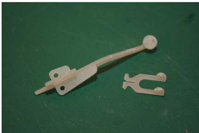
**2.41.4** The tail wheel runs on an axle of 1.5mm carbon rod. Before fitting this though it's best to paint the assembly and the wheel centre to your preferred colour
