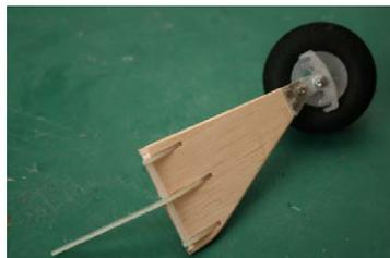
plate, followed by another washer, spring washer and nut to lock the axle to the axle plate. See the notes on the drawing. The spats, if you are using them, can be fitted later. Then it may be necessary to adjust the number of washers to get the best clearance between the wheel and the inside of the spat.
