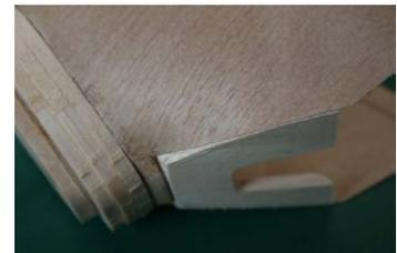
Swann Morton with a No26 or No23 blade), a razor plane, or (initially) a very coarse sanding block. Or all three. Start by shaping the sides to the angle of the cowl MC1, moving slowly down the side to the undersurface where the angles get quite steep. Do small amounts at a time,
