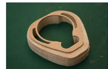
leave to set with a weight upon it. Then glue MC5 to MC4. Resin or slow cyano is fine, (needs to be a glue that will carve and sand easily, so NOT epoxy), but do ensure that all the parts stay in perfect alignment – use
