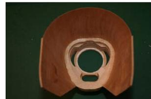
**2.43.8** Mark out the upper and lower edges of MC9 as diagram on drawing. The lower front edge has to be chamfered to the line so that it butts up to the rear of MC2 at the correct angle, and the sides so that they fit inside MC1, though the side chamfer is reduced to the rear. The upper rear surface
