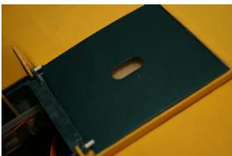
**2.44.3** FB5 fits by sliding it rearwards so that its tab engages under the rear edge of FB2, (which isn't fitted yet but is just about to
