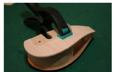
the edge off your scalpel or razor plane blade. It is likely that SP4 and SP5 are not exactly the same thickness, so once the SP4's are dry, place that face on a sheet of sandpaper and sand it flush all over to accept the next lamination.
