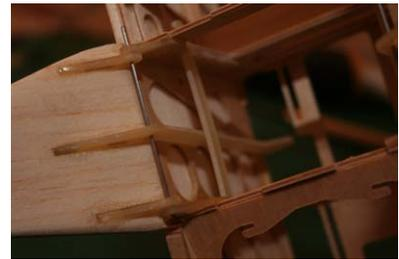
**2.45.10** Repeat for the other leg. Use a rubber band stretched between the rear ends of UC6 - notches are provided for this - to secure them in position.
