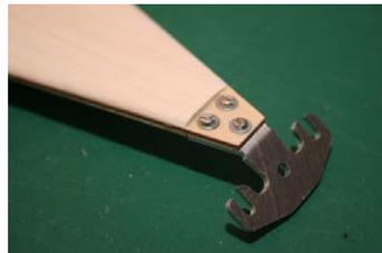
**2.45.7** At the top of each leg, on the outside, sand a small chamfer. *However, on the inside sand a much bigger chamfer down to the ply core, particularly on the short edges outside the pivot plates - this last is important to allow the legs to settle into alignment when you fix the legs into position on the UC5's. See pictures section 2.45.4 on previous page.*
