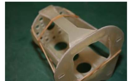
**2.51.7** Insert the motor through the back of the mount and fix it to the front plate according to the instructions that came with it. Use lock-washers under the bolt heads and make sure the bolts are not so long that they foul the coils within.
