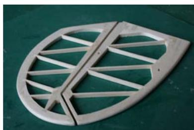
**2.50.9** Now for a bit of wooden engineering ... Cut out the ply 'V' brace TS1, the ply trunnion pairs TS2, (four per V brace), and the epoxy glass trunnions TS5. Bush the TS2's with the 2mm tube, which you may find easier to do while the parts are still retained in the mother sheet. Spares are provided since these small parts are easily lost!
