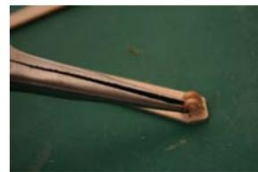
ideal for positioning the trunnions into the V brace slots. Repeat for the other one, making sure – very sure – that it is the opposite hand. Note the small hole just below
