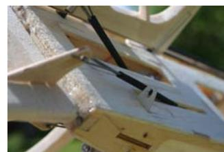
across the upper surface of FB4b. Make very sure it is positioned centrally, then bond in place with thin cyano or epoxy.
