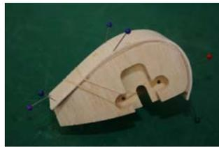
**2.46.13** Build up the next layers, making sure for each layer that the join line between the longer and shorter sections is sanded flush and smooth before adding the next layer.
