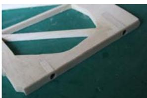
**2.50.5** Sand lightly both sides, and plane/sand the leading edge to section. Remember to mark the centre of the leading edge, as with the rudder, so that as you sand it you keep the upper and lower profiles the same. (See GNF234-2 for section sketch). Then
