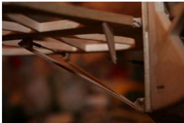
**2.50.14** Repeat for the other side. Make sure the stabs are pushed firmly home against the fuselage, and then nip up the nuts, which will clamp the epoxy glass trunnions TS5 to TS4. This will firmly locate the stabiliser.
