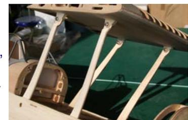
2.47.3 The cabanes are faced only on the outside with balsa CB1a and CB2a, but these must be laminated only after the upper central wing section is made and fitted. See Section 3. The lower edges of the facings sit down on FT1 just inside FS1. Damp them well to assist
