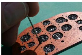
**2.49.1.2** There are holes drilled along the bottom of the dashboard, if you wish you can insert into these small pins with the heads cut off to represent switches, knobs etc.
