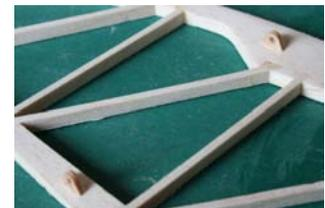
**2.50.6** Proceed with the elevators in the same way, with the outline set by parts E1 ~ E6, and the diagonals E7 ~ E12. As usual, sand both sides very lightly, and draw a light guide line at half-thickness around the rear and side edges. Reinforce the inside
