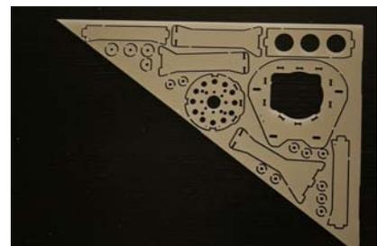
**2.51.5** It pays to practice the assembly of the parts a few times so that when you come to finally epoxy it all together you won't get into too much of a sticky mess. First of all - note that the Back Plate EM35BP and the Front Plate EM35FP each have two small witness holes drilled in one of their sides. When assembling the parts
