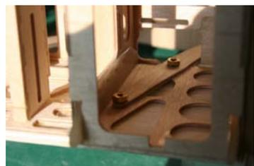
2.47.2 The front hatch will now be quite tricky to fit since the upper central wing section is not fitted yet. When it is, the cabanes are splayed outwards into a gentle 'S' shape when viewed from the front, which gives more clearance to fit the hatch.
