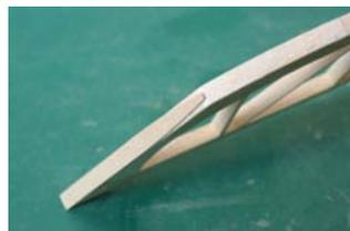
angled edge with ply part E13. Taper the trailing edge similarly as for the rudder, and E13 will make a useful template. Use a long sanding block to cover
