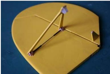
**2.50.13** Remount the tail and fix the inner end of TS1 to TS4 with an M2x8 bolt. Thread the bolt through from the front, and *loosely* fasten with a lockwasher and nut. Note that TS4 has an oval hole to allow for the tightest adjustment .
