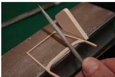
**2.48.3** The side screen front pillar fits on the side of the main screen side pillar, (not behind it), so the sides of the main screen need to be chamfered as shown on the
