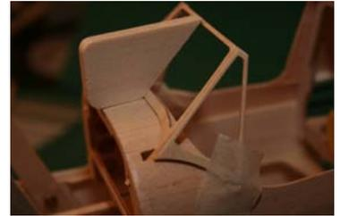
**2.48.4** When you are happy and have made a port and starboard side, with the main frame inserted glue the side frames to it with resin taking care to line up the front edges of the side screens and main screen and also not to bond any part of the screen to the deck at this stage. When set, remove the assembly and carefully round off the outside front edges.
