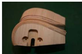
**2.46.15** A further refinement of the above, if you're happy using slow cyano, is to use the cyano just around the forward tightly curved section. (Still dampen the balsa of course). Then brush resin over the rest of the joint, pull it tightly to the end, invert it and clamp with a heavy weight as mentioned above in 2.46.12.
