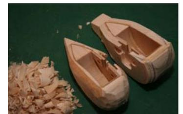
Now is the time to switch to using coarse sandpaper, (say 60 grit) to start getting the profile even better. Check the view from the front, the back, and all angles in between as you work, to make sure that the spat shape stays symmetrical.
