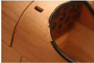
**2.48.7** Once all that is dry, fit the sidescreen infills. Sand off any projections beyond the face of F4a, so the hatch will fit closely to it.
