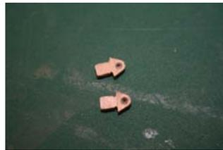
bush the holes in the two ply trunnions TS3 with 2mm plastic tube, and fit them into the slots from the underneath of each stab half. The TS3's will be a firm fit in the stab, and could be glued in place, but you may find it easier to cover the stabs if this is left until after covering. That completes the stabs for now.
