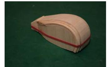
**2.46.17** May we suggest, (having done it a few times), the following: Using the ply guide SP18, draw around it on the top and the bottom. Also draw a line down the centre. Use a razor saw, razor plane or a No26 scalpel to
