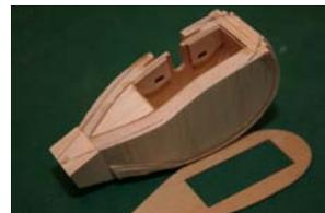
shape the spat working from the centre of each side towards each end until close to the guide lines. Now, working from the centre top, and looking from the front,
