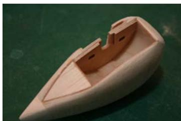
2.46.19 Take two 2.5mm x 8mm bolts (per spat) and file the head as shown on the drawing GNF234-2. Install the bolt from the inside of the spat, and epoxy in place. When dry,
