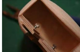
you will be able to slide the spat bolts into the slots of the axle plate, and lock in place with spring washers and a nut. An M2.5 nut-runner is really useful for this job.
