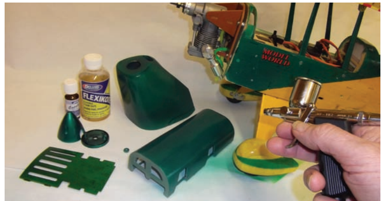
All the green components and fuselage front end were sprayed with Auto-Air Colours paint, and then fuel-proofed with FlexiKote
