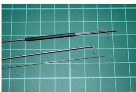
1.4 mm rudder pull-pull wires are straightforward 90-degree bends with 0.6 mm retaining wire
