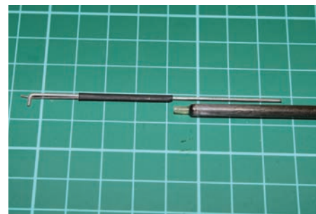
Elevator pushrod servo end; note the rounded off carbon tube
