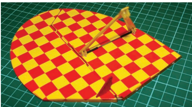
Underside of one tailplane half and the strut is now fitted; note the plywood horn has been painted to match the scheme
