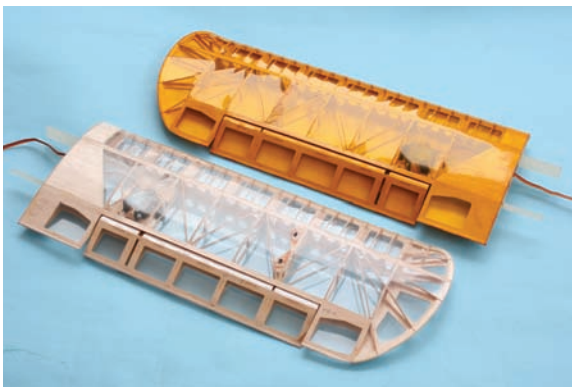
It was finally decided to change the clear transparent film finish to a coloured transparent scheme
