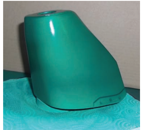
With several coats of Poly-C and sanding, the sprayed finish looks perfect
