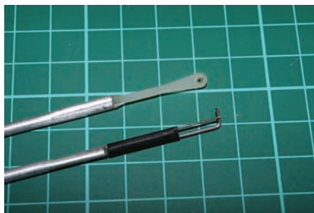
Aileron pushrod with lower wing connection shown with the hole and tube bearing, with the top wing connection shown below
