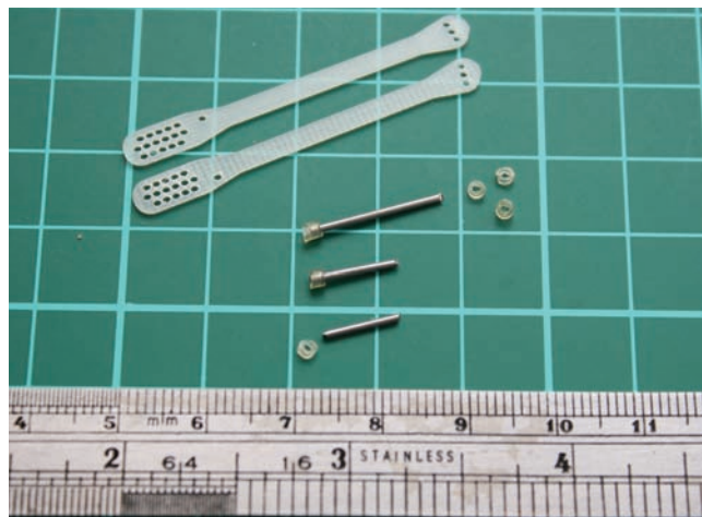
The aileron pushrod is made from two identical fibreglass pieces with adjustment holes; 1 mm wire pins are made up to secure the pushrod
