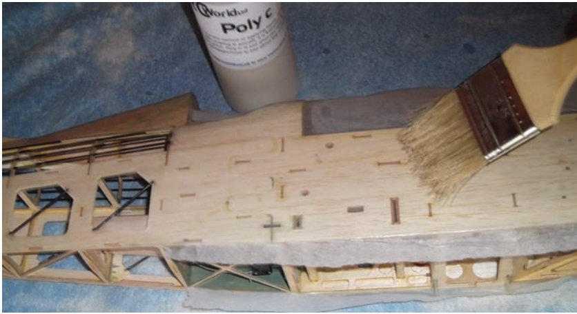
With tissue applied, several coats of Poly-C were brushed onto the fuselage to give a smooth finish
