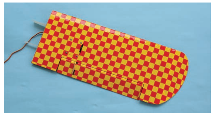
Undersides of the flying surfaces were covered with chequered Oracover, and the pattern match was fairly easy to achieve
